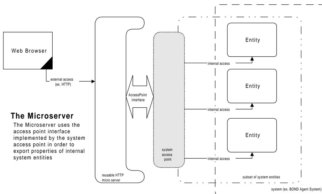
Both accesspoints discover object properties, fields and methods (i.e. without involving the Object's code itself) by use of the java reflection mechanisms. In this respect the accesspoints can be reused as "observers" within any system.
