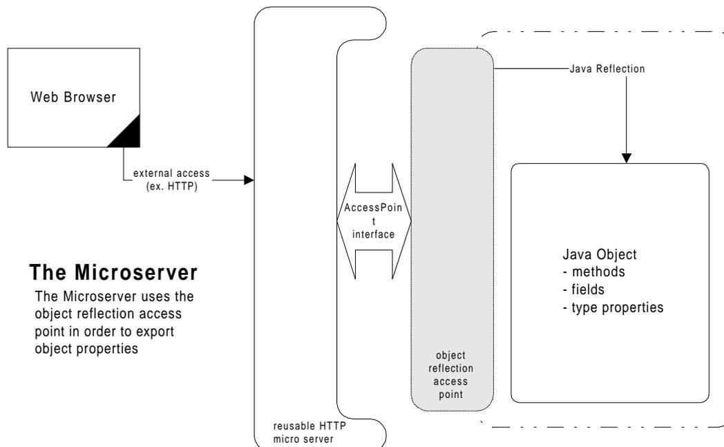
As can be seen from the figure, the accesspoint actually *wraps* an associated Object and uses internal access mechanisms (i.e. method calls). The example java source code associated with the above figure would be:
