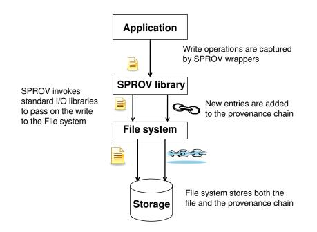
Fig. 4. The Sprov System Architecture.
