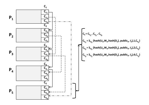
Fig. 3. Example of a spiral provenance chain with R = 3, i.e., 3 checksums per provenance entry. For example  $P_5$ 's checksum  $C_5$  has 3 separate checksums in it. Each checksum is computed by concatenating the hash of the current content of  $P_5$  with a checksum from a previous entry. In the example,  $C_{5_1}$ ,  $C_{5_2}$ , and  $C_{5_3}$  are computed using  $C_{4_1}$ ,  $C_{3_2}$ , and  $C_{1_3}$  respectively.
