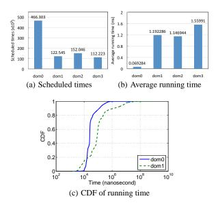
Figure 3: Motivating example. (a) Scheduled times for each domain in 5 minutes. (b) Average run time for each domain in 5 minutes; (c) CDF of running time for dom0 and dom1.
