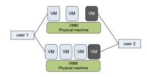
Figure 1: Multiple MapReduce clusters deployed in a virtualized data center. VMs with the same shade belong to one cluster.
