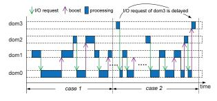
Figure 4: Excerpt of the trace file of domain scheduling. Case 1: interleaving of domains issuing I/O requests; case 2: delayed execution (I/O request of dom3 is delayed by dom1 and 2.)
