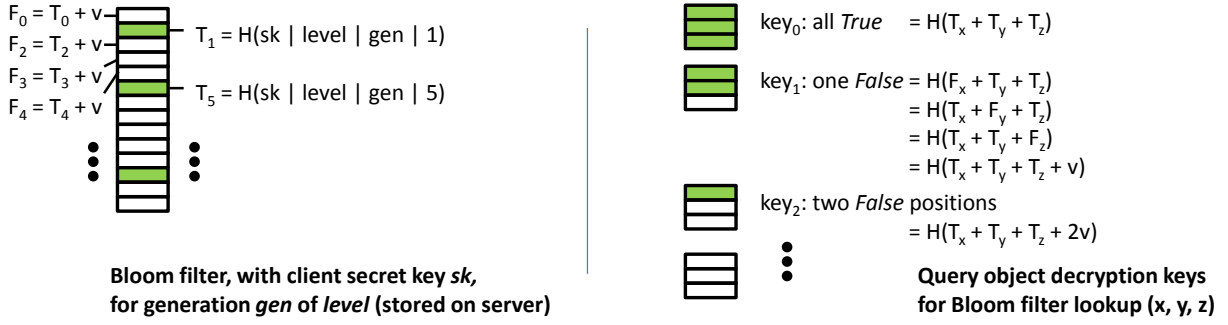
Figure 3: Left: Bloom filter format in full construction. A bit set to 1 in the Bloom filter is represented by a hash of the position and current level key; a bit set to 0 is represented by the same value, plus the secret value v . Right: decryption keys used with the query object. The server obtains the decryption key for a given query stage by hashing together the specified Bloom filter results. Since there are k hash functions used in a Bloom filter check, the client includes in the query object an edge corresponding to each of the k + 1 possible keys.
